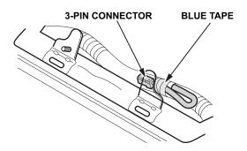
Slide the transceiver onto the antenna bracket as shown.
