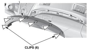
5. Remove the driver's dashboard lower cover. NOTE: To avoid whitening the dashboard cover, start by gently and evenly pulling out on the lower edge of the cover to release its lower clips, then work your way up the cover to release the middle and top clips.
